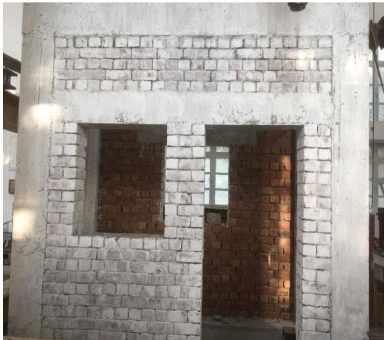
Figure 3.2 Reinforced concrete infill wall frame with window and door opening fabricated in lab
