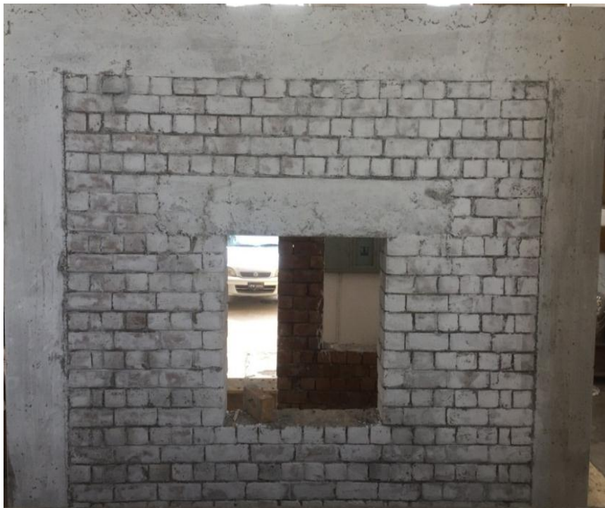
Figure 3.4 Reinforced concrete infill wall frame with window opening fabricated in lab
