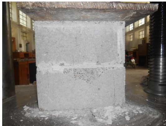
Figure 1: Testing of concrete block masonry units under compression using universal testing machine
