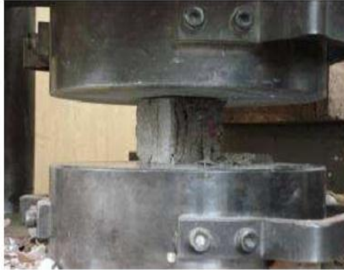
Figure 2: Mortar cubes under compression test
