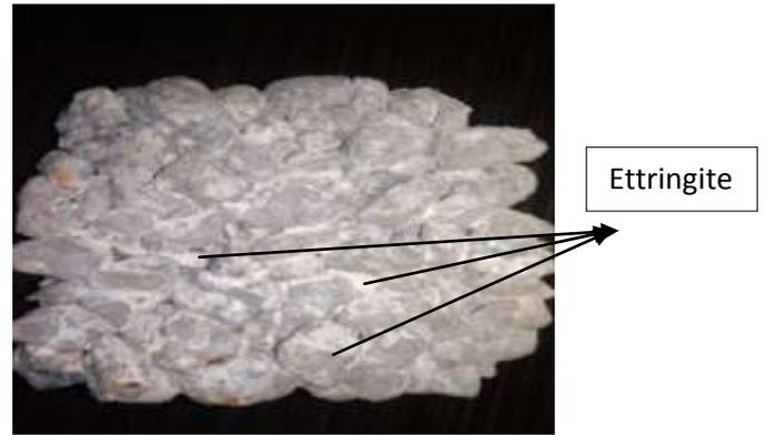
Fig. 12: Cube after sulfate attack
