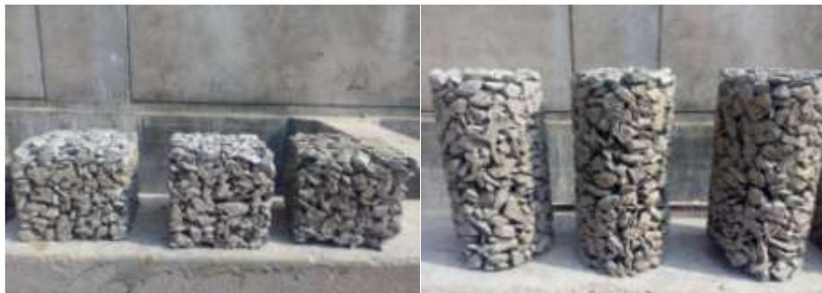
Fig. 1: Pervious concrete specimens of cubes and cylinders
