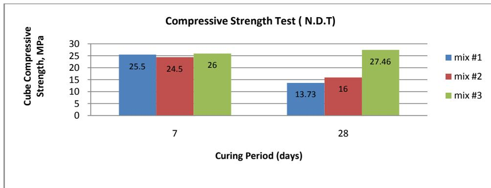
Fig. 5: Compressive strength (N.D.T) Vs curing period
