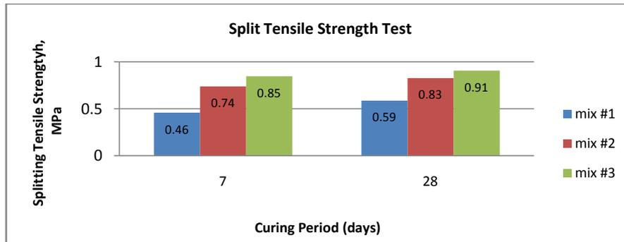
Fig. 6: Split Tensile Strength Vs Curing Period
