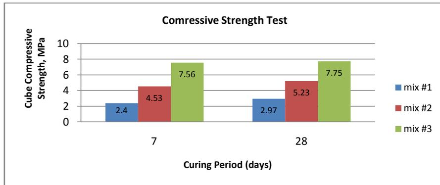
Fig. 3: Compressive strength Vs curing period
