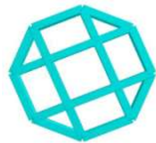
Octagonal & Plus Bracing
