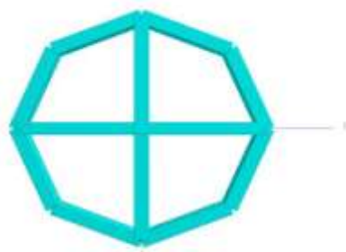
Octagonal & Cross Bracing
