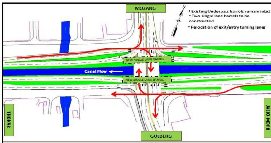
Figure 5. Diagrammatic Representation of Option-II
