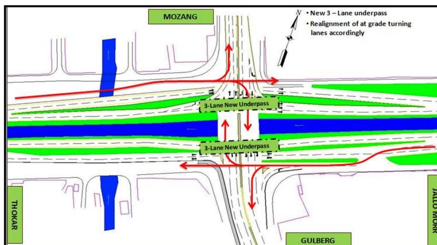
Figure 6. Diagrammatic Representation of Option-III
