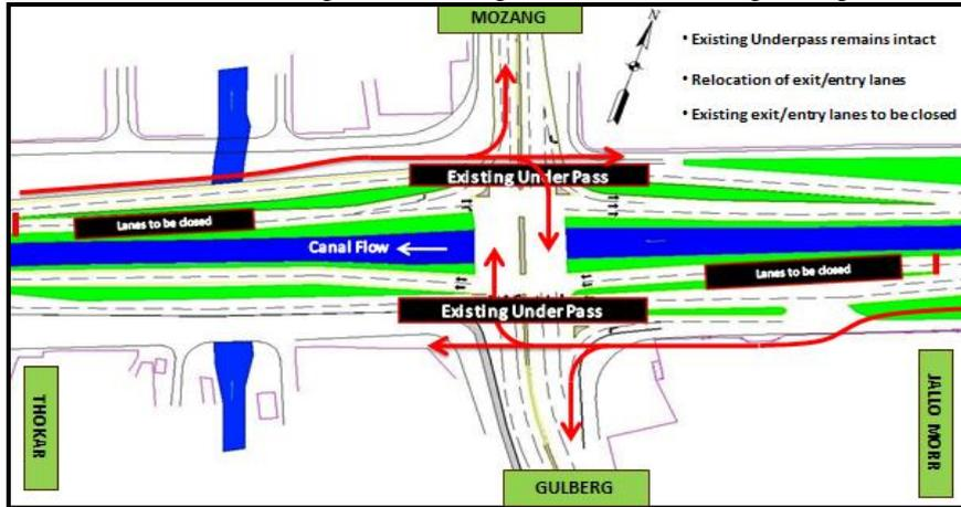
Figure 4. Diagrammatic Representation of Option-I
