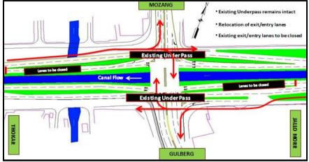
Figure 4. Diagrammatic Representation of Option-I
