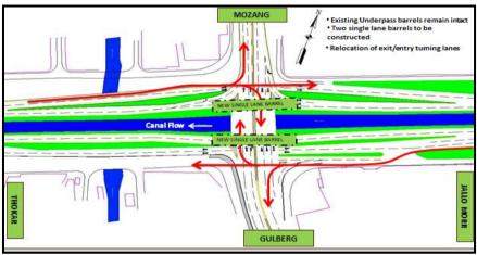
Figure 5. Diagrammatic Representation of Option-I
