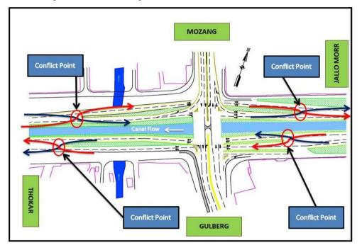
Figure 2. Traffic Weaving Phenomenon at Jail Road Underpass
