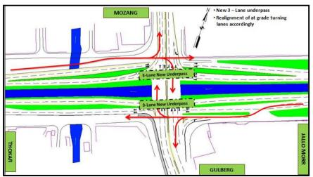
Figure 6. Diagrammatic Representation of Option-III
