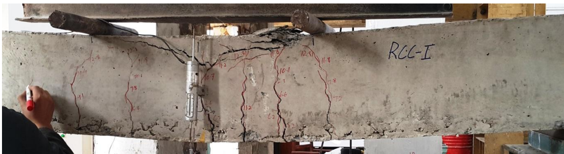
Figure – VI (a) Crack pattern of RC beams in failure at 12.8 Ton
