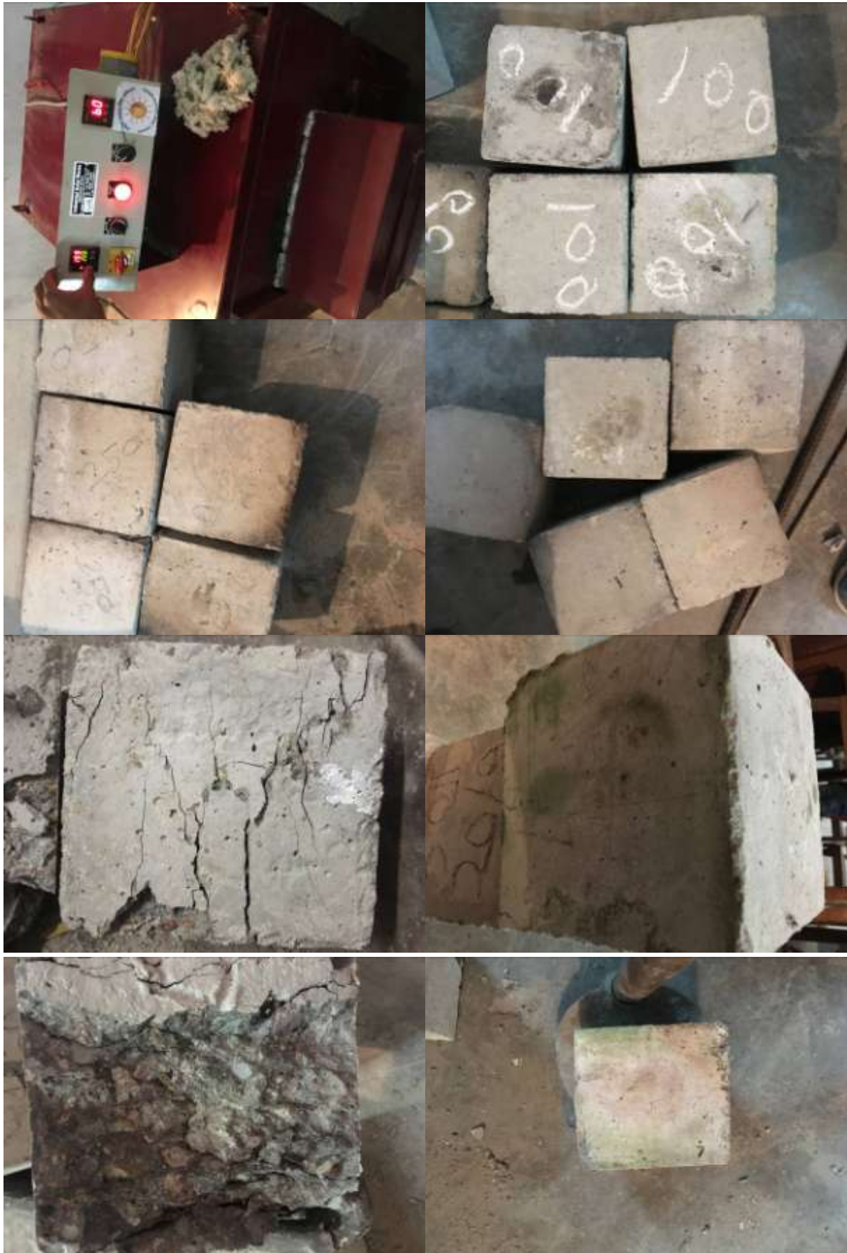
Fig-1-6 Furnace, Samples at 100/250/500C, Failure pattern and change in color.
