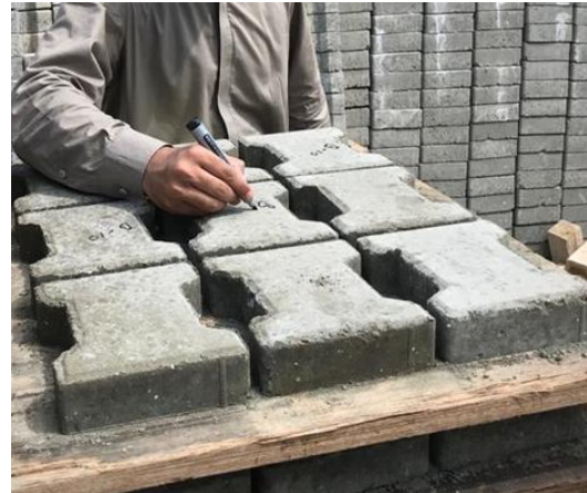
Proper tagging and marking of paving blocks after casting
