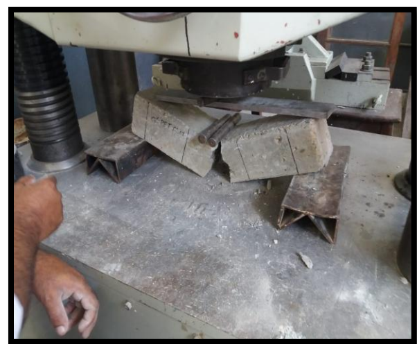
Figure 6 Testing of Samples for Flexure Tensile Strength Test
