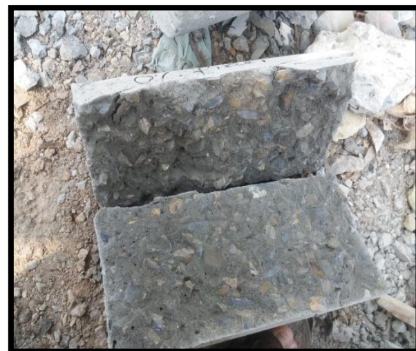
Figure 5 Testing of Samples for Splitting Tensile Strength
