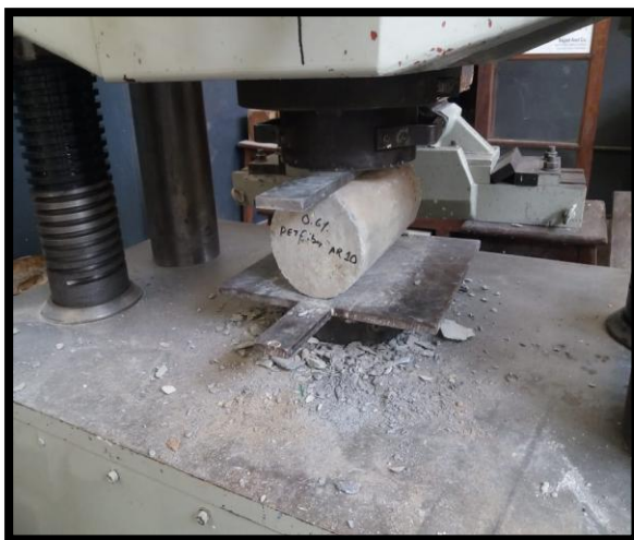
Figure 5 Testing of Samples for Splitting Tensile Strength
