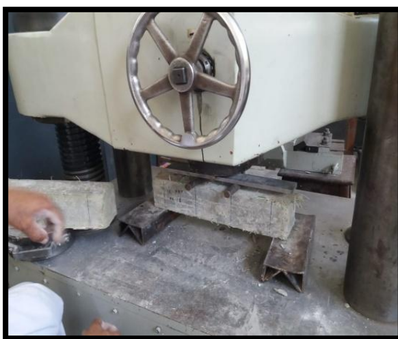
Figure 6 Testing of Samples for Flexure Tensile Strength Test
