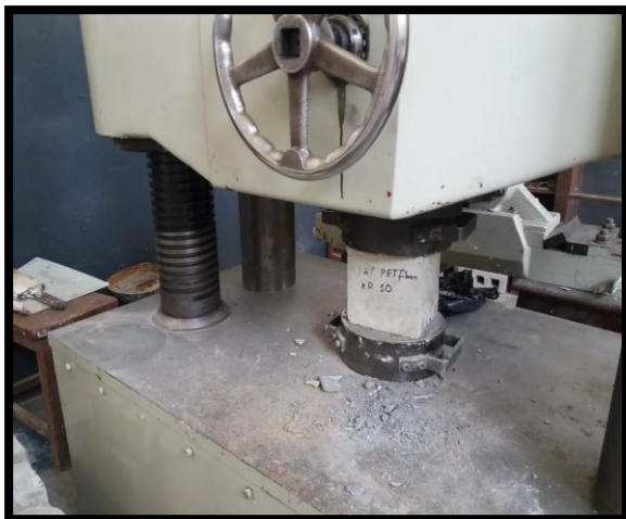
Figure 4 Concrete cubes Samples Testing
