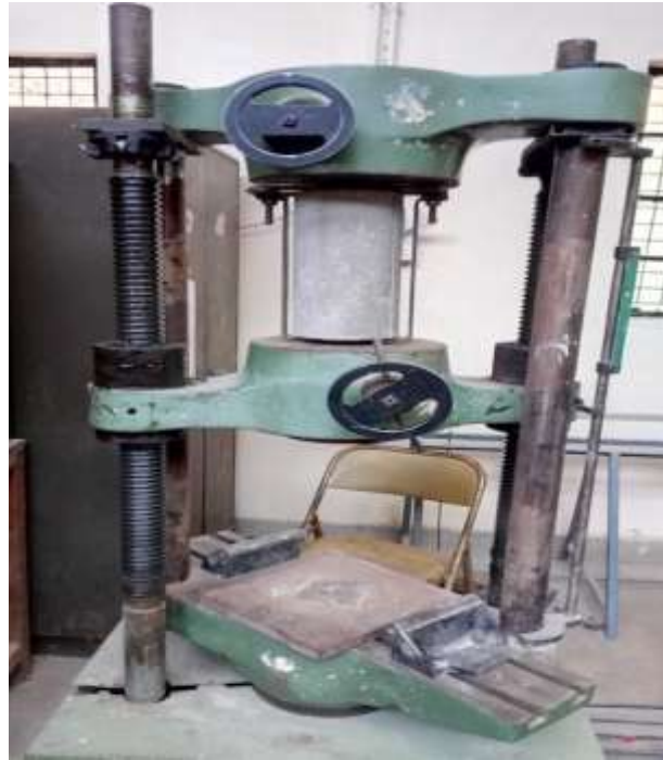
Figure 5. Bond strength test setup
