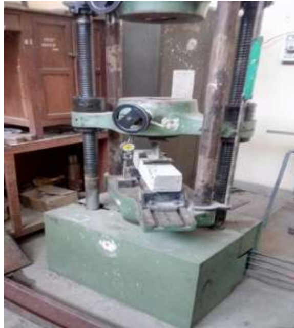
Figure 6. Flexural strength test setup
