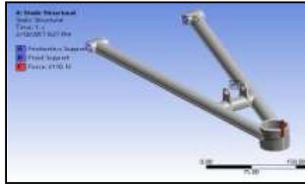
Figure 6. Boundary condition for A-arm
