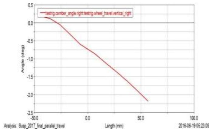
Figure 4. Camber Vs Wheel travel graph.
