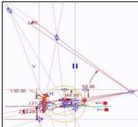
**Figure 2. ICR diagram of suspension system**
