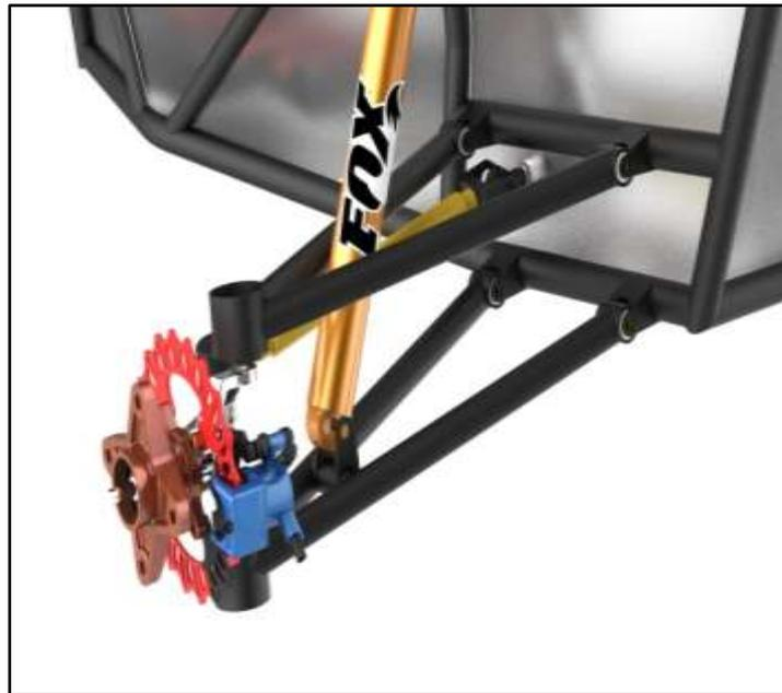
**Figure 1. Double Wishbone Suspension system**
