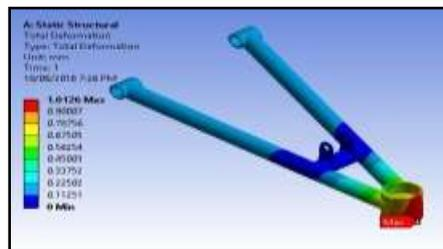
Figure 8. Deformation of A-arm
