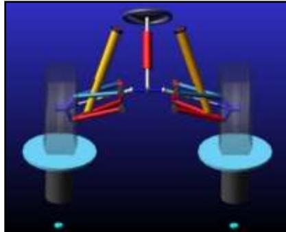
Figure 3. Simulation of front suspension on MSC Adams
