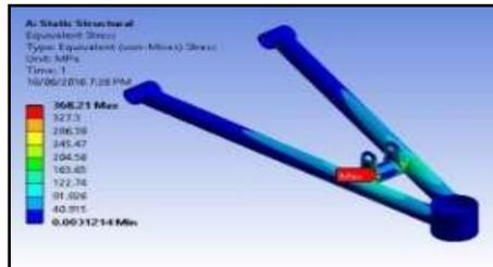
Figure 7. Von mises stress in A-arm
