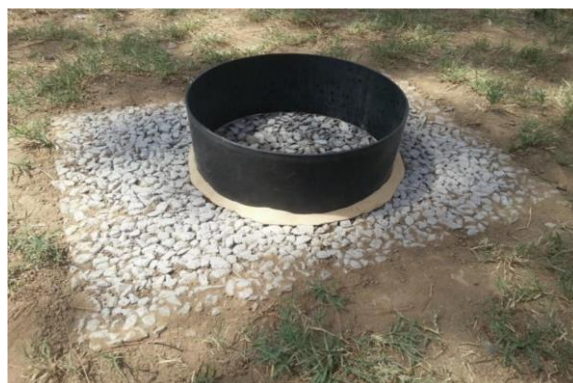
Figure 7: Infiltration test performed on pervious concrete on site
