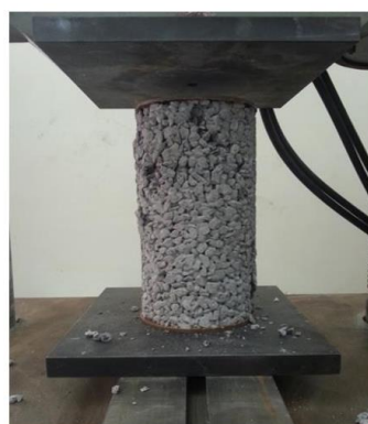
Figure 2: Figure shows testing of cylinder specimen in UTM
