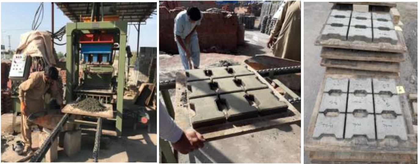
Proper tagging and marking of paving blocks after casting
