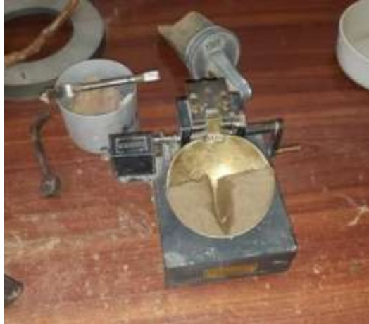
Figure 2: Cassagrande apparatus for liquid limit test
