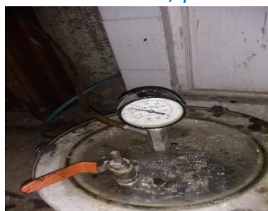
Figure 5. Application of vacuum
