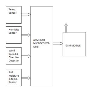
Fig. 1 basic block diagram of proposed system
