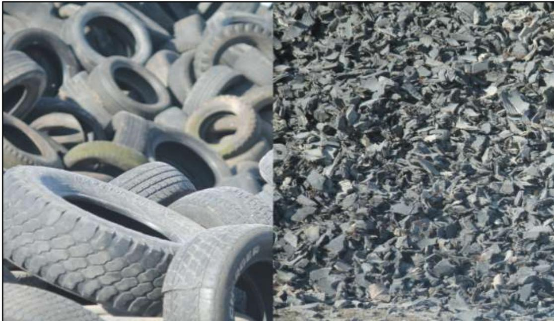
Figure 1. Tire derived aggregates (TDA)
