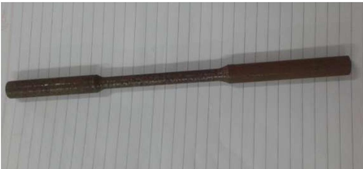
**(Figure 4. Specimen rod of Material SAE8620)**
