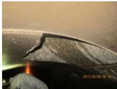
Figure 12: Pipe fracture at the joints
