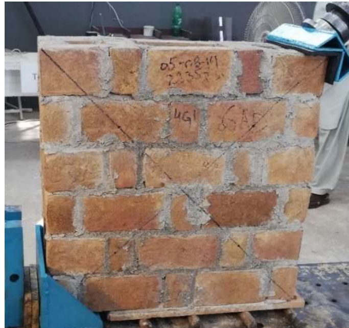
Figure 6. Testing arrangements for diagonal shear strength test
