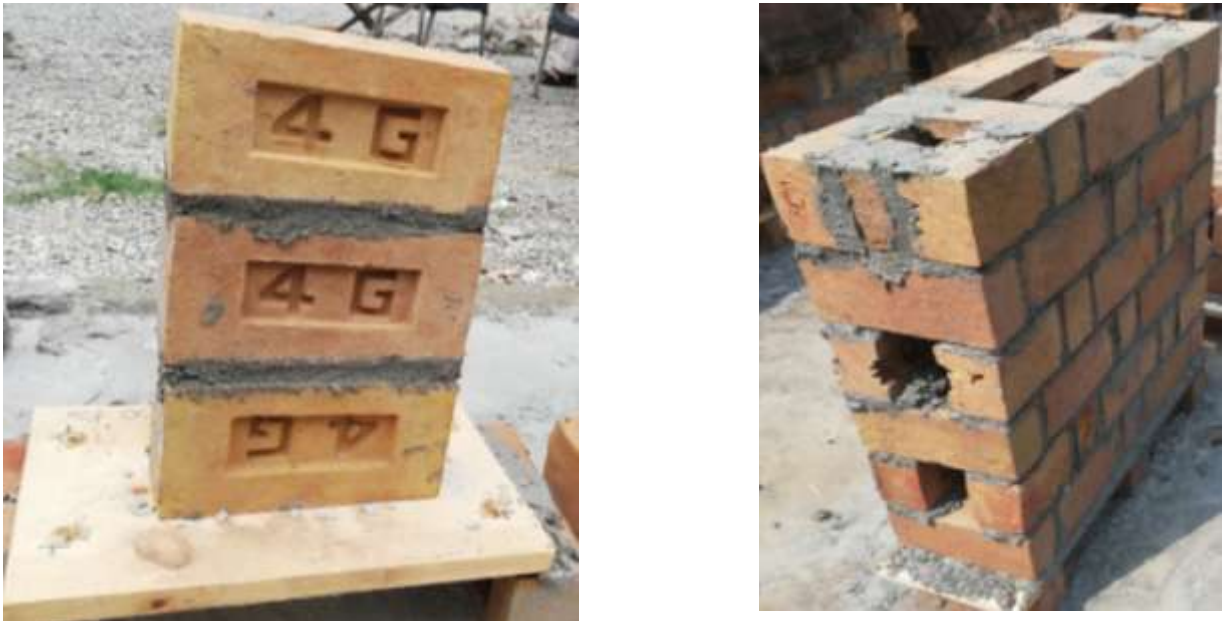
Figure 4. RTB testing Specimens Triplet and diagonal prism
