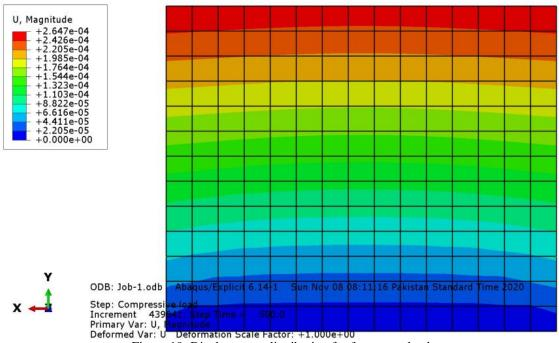
Figure 10: Displacement distribution for four-story load
