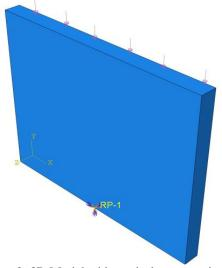
Figure 2: 3D Model with vertical compressive load and B.C
