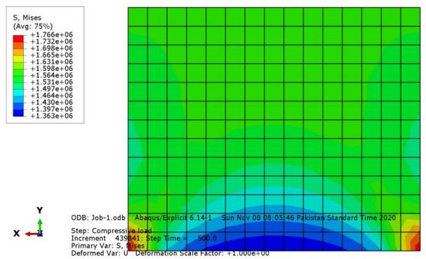
Figure 7: Von-Misses stresses for three-story load
