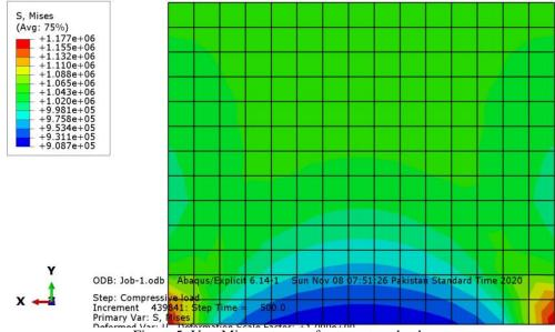
Figure 5: Von-Misses stresses for two-story load
