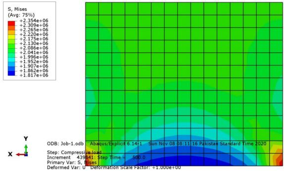
Figure 9: Von-Misses stresses for four-story load
