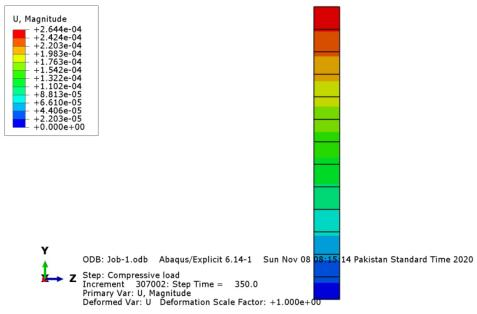
Figure 11: Side View of the wall (no lateral displacement)
