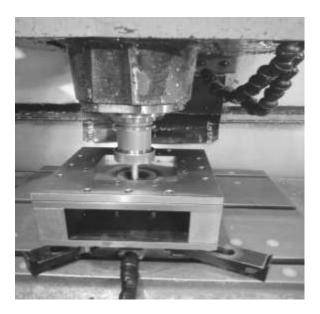
Fig 1.Incremental sheet metal forming process [5]
