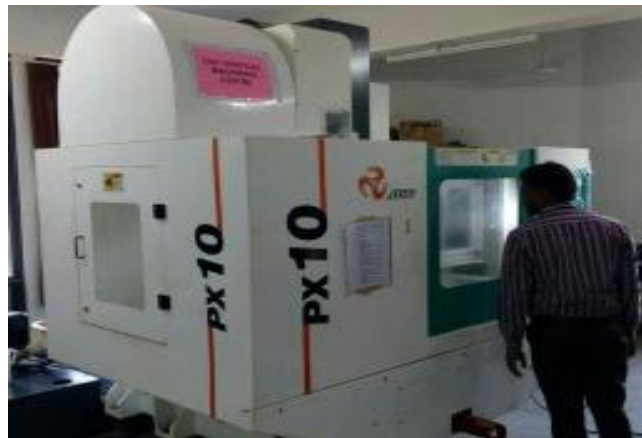
Figure 2 CNC Vertical Milling machine used in Experiment for drilling
