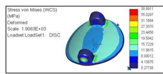
Figure 9(c) Von mises stress acting on valve disc
