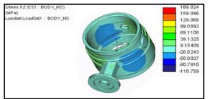
Figure 8(c) Hoop stress acting on valve body
