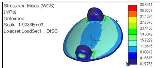
Figure 9(c) Von mises stress acting on valve disc
