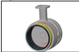
*Figure 5(a) Seat molded to valve body*
