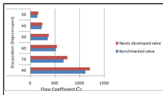
**Figure 10(c) Flow co efficient at different angles of disc opening**
