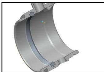
*Figure 6(a) Seat assembly in body*
