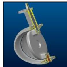
Figure 3(b) Sectional view of butterfly valve.
