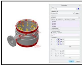
Figure 8(a) Body is constrained in all DOF
