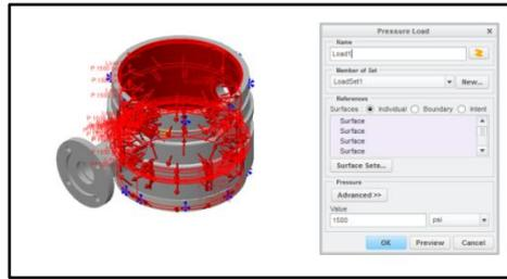
Figure 8(b) Pressure applied on valve body
