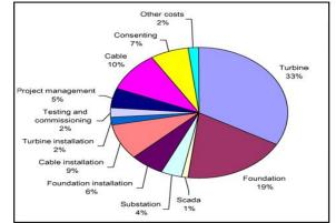
Figure 6: Estimation of capital cost for an offshore wind farm.
