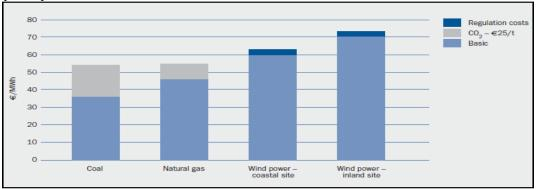
Figure 4: Cost of generated power as compare to conventional power plants
