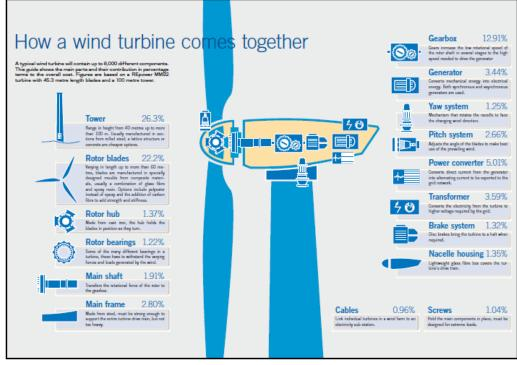
Fig. 2. The main components of a WTG set and their share to the overall cost (for the 05 MW RE Power machine)
