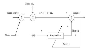
Fig2. ANC with uncorrelated noise m<sub>0</sub> in primary input
