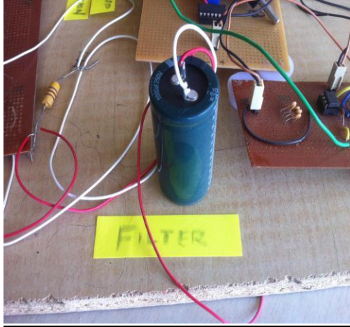
Fig: 3(a) Filter Capacitor.
