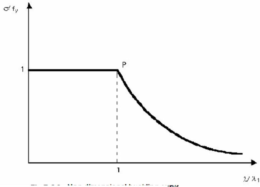
Fig.3: Non-dimensional buckling curve
