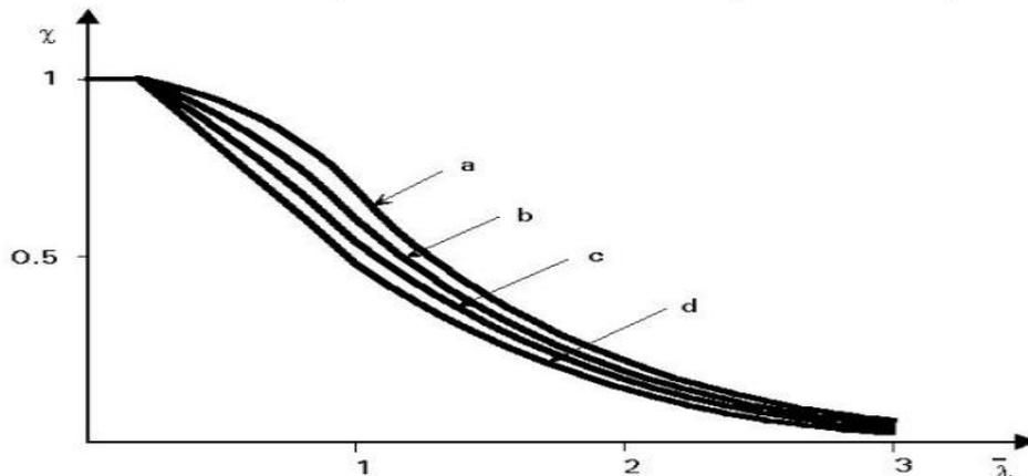
Fig. 8: European buckling curve
