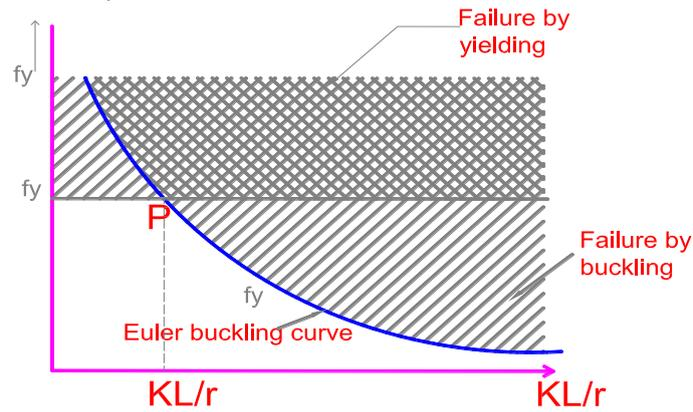
**Fig..2: Local buckling curve and modes of failure**
