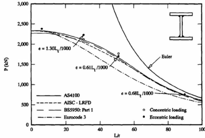
Fig. 7: Comparison of design strengths and test strengths for I section columns using nominal values
