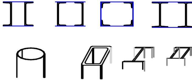
Fig. 1: Cross sections of compression members
