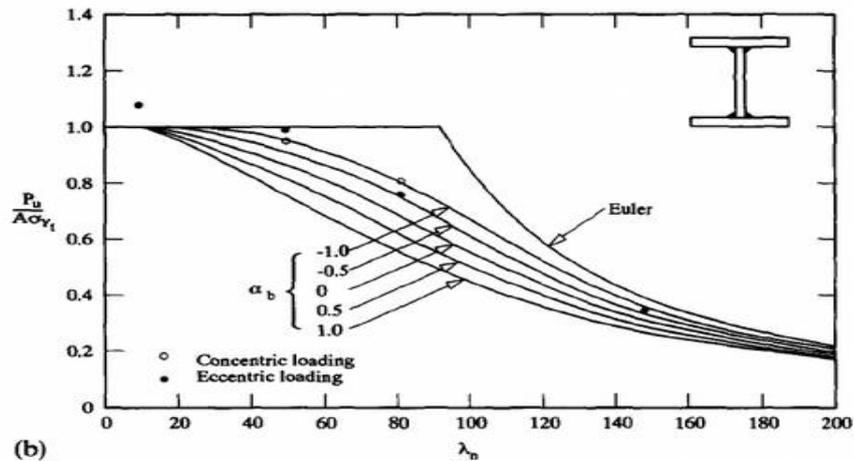
Fig. 9: Column curves of AS4100 for I section columns
