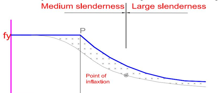
Fig.4: Real column test result and buckling curves
