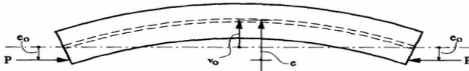
Fig. 5: Loading eccentricity and geometric imperfection
