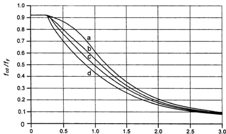
**Fig. 6: Column buckling curve**
