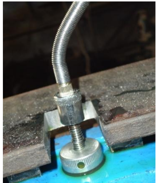
Figure 8. Thermocouple at side and top on gear casing.
