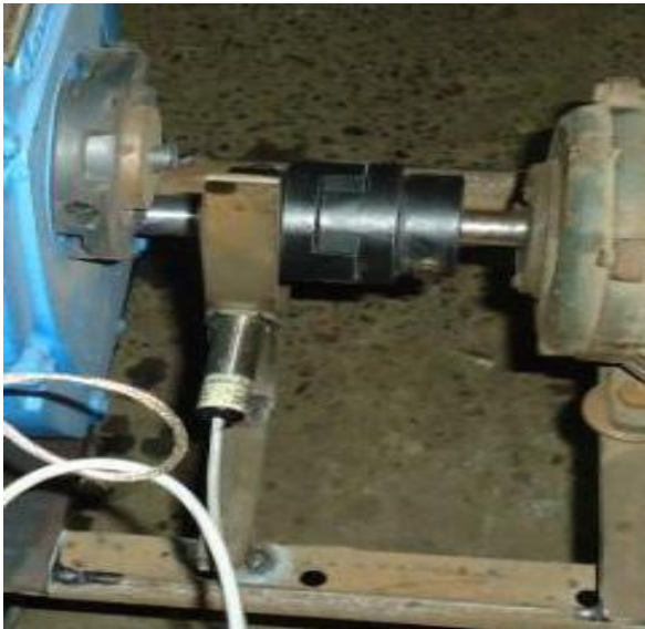
Figure 5. Proximity sensor at input and output shaft.
