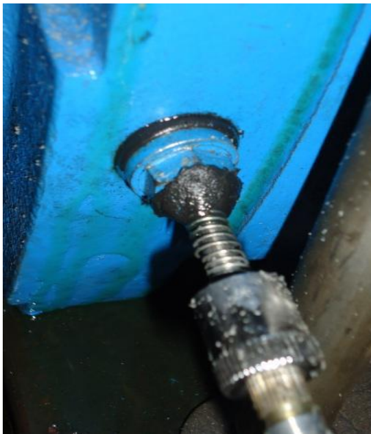
Figure 8. Thermocouple at side and top on gear casing.
