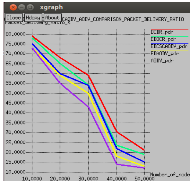
Figure 3 Comparison of DCDR, EDAODV, EDCSCAODV, AODV and EDOCR on the basis of packet delivery ratio
