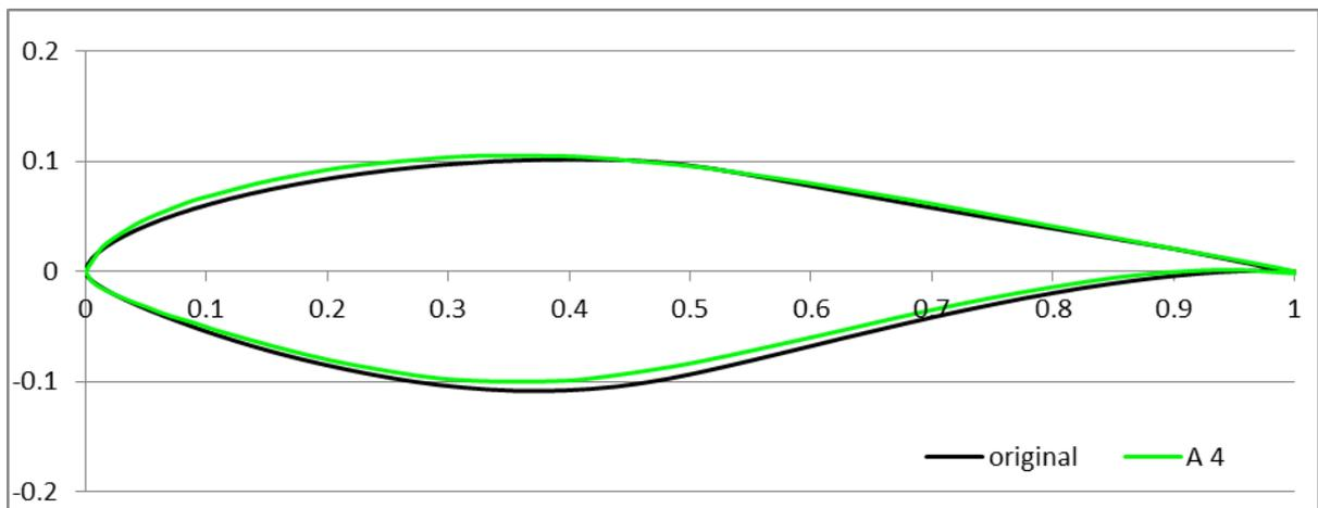
Figure 7. Comparison of shape of A4 individual with original airfoil.
