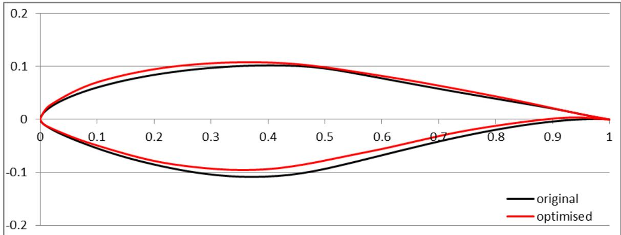
Figure 8. Comparison of shape of optimized airfoil with original airfoil.
