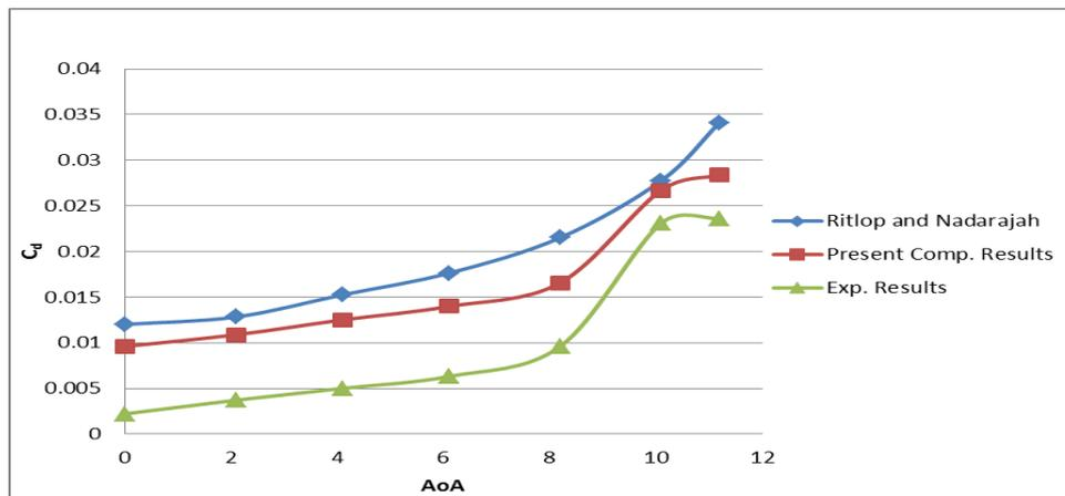
Figure 3. Variation of drag coefficient with angle of attack
