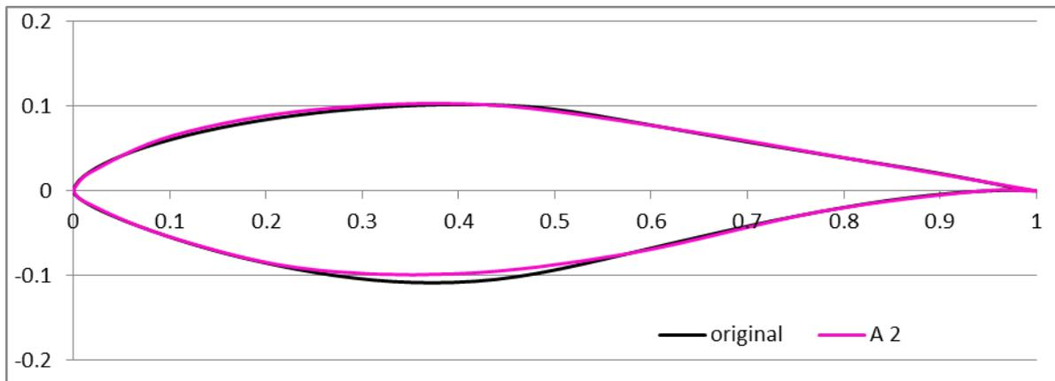
Figure 5. Comparison of shape of A2 individual with original airfoil.
