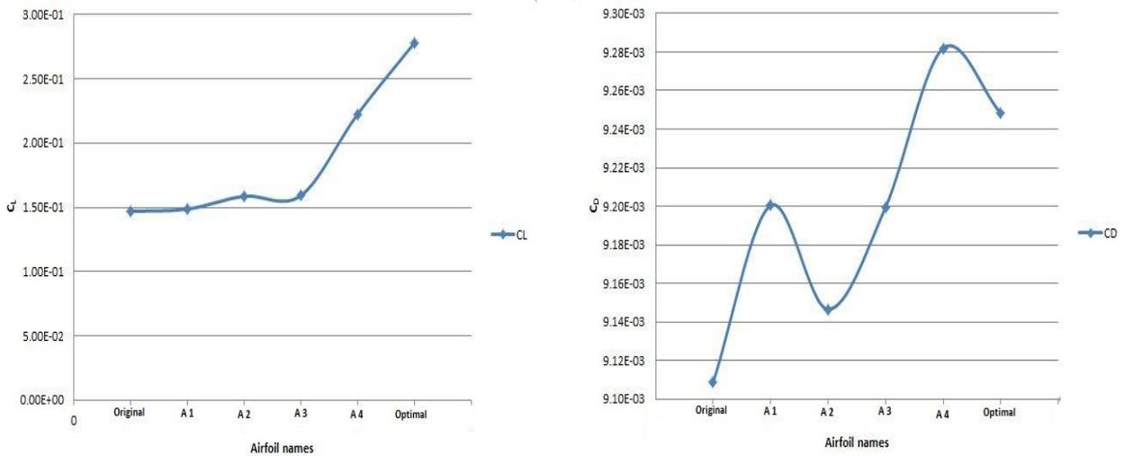
Figure 10. Comparison of Lift ( $C_L$ ) and Drag ( $C_D$ ) coefficients.
