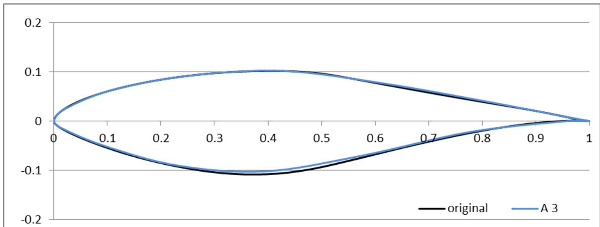
Figure 6. Comparison of shape of A3 individual with original airfoil.
