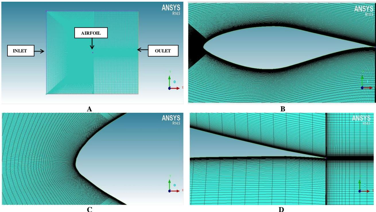
Figure 1. A) Mesh domain. B) Refined mesh near wall. C) Mesh near leading edge. D) Mesh near trailing edge.
