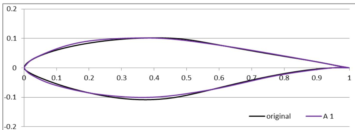
**Figure 4. Comparison of shape of A1 individual with original airfoil.**
