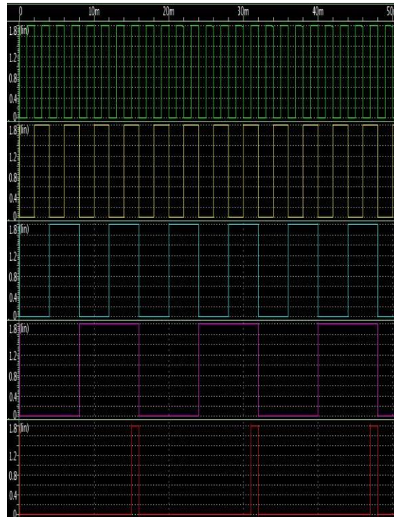
Figure 8 Waveform of 4-bit AND gate
