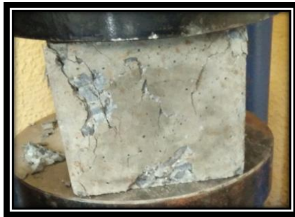
Figure 2: Tested Sample of M30 of concrete
