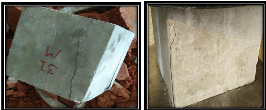
Figure 4: Tested sample of Micro concrete
