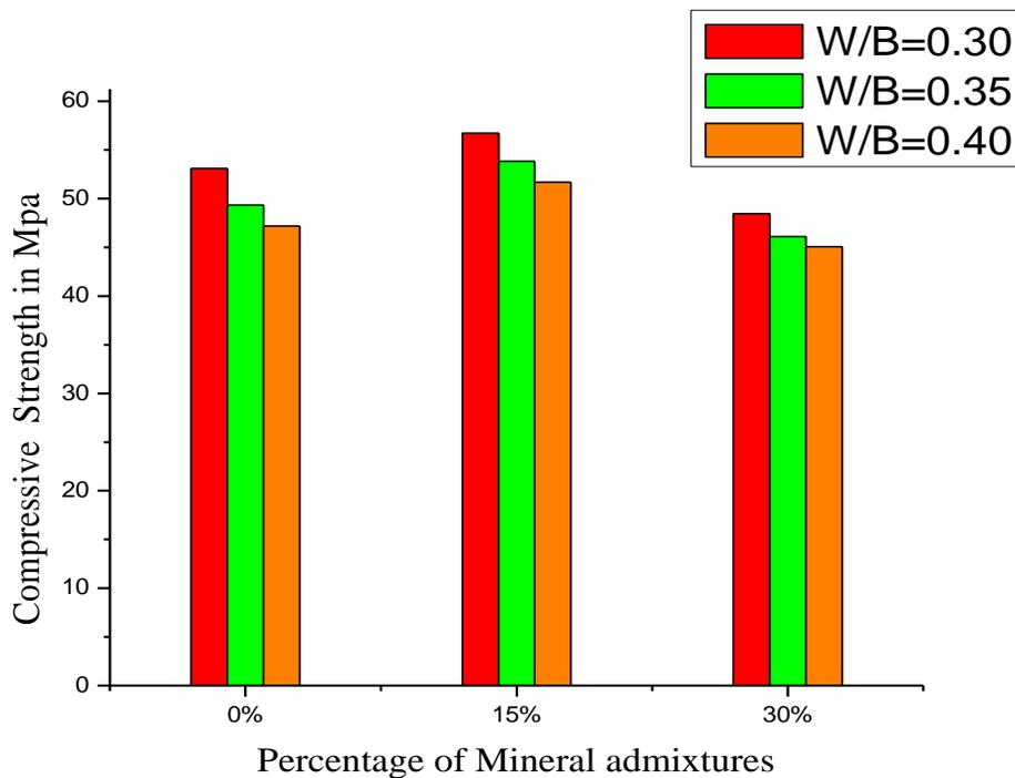
**Figure 3: Compressive-strength for Partial replacement of cement with (0%,15%,30%) of mineral admixtures for 1% fibers (0.75% S.F & 0.25% P.F) for 28 days**
