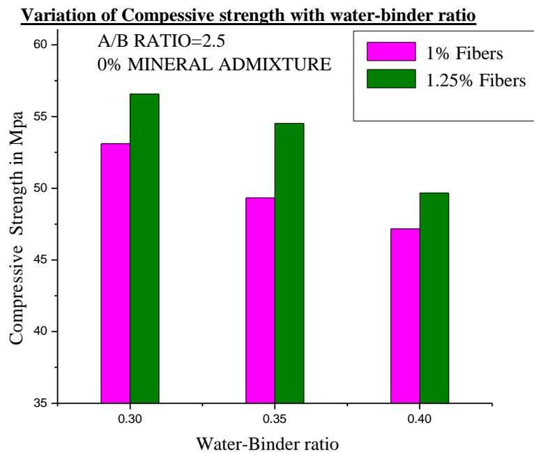
Figure 6: Compressive-strength vs. Water-Binder ratio with different fibers percentage with 0% mineral admixture for 7 days
