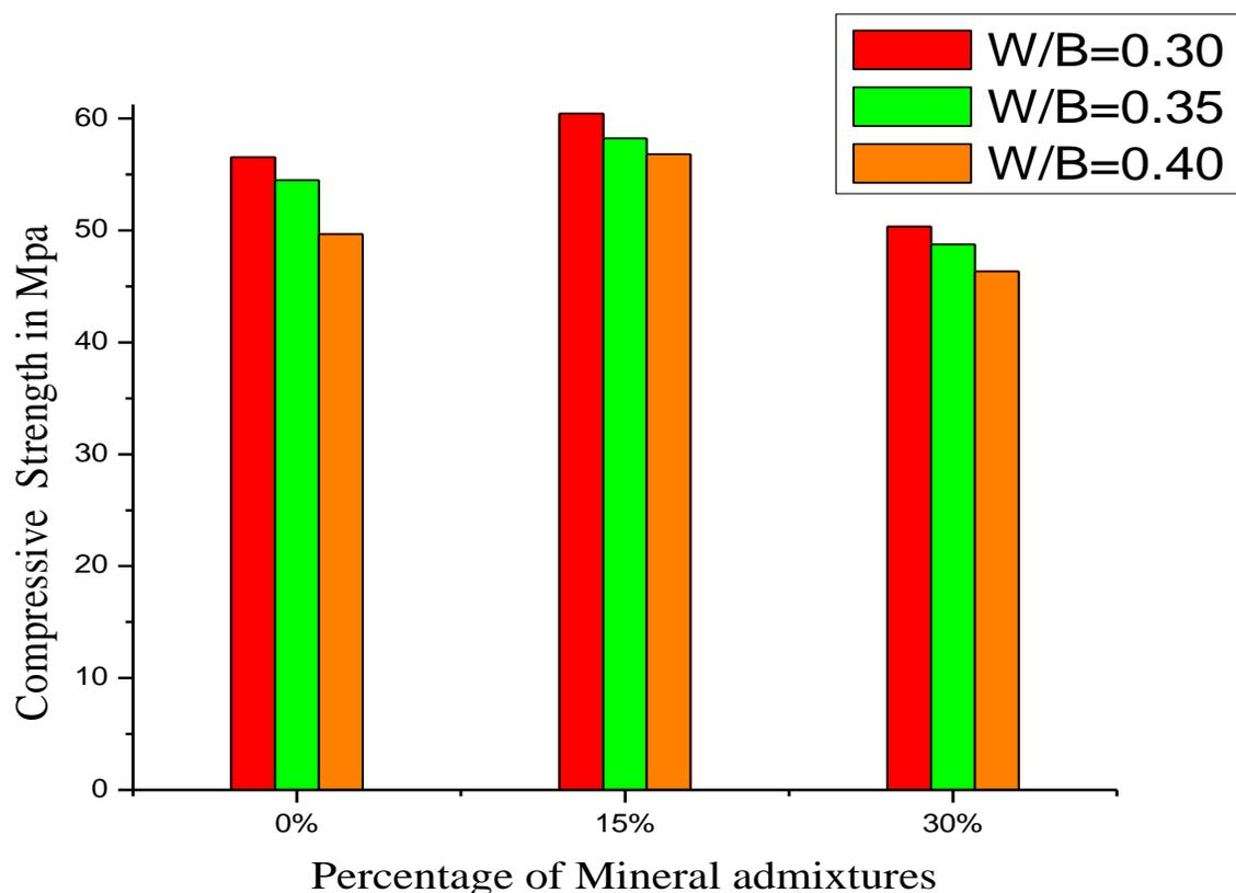
**Figure 4: Compressive-strength for Partial replacement of cement with (0%, 15%,30%) of mineral admixtures for 1.25% fibers (1% S.F & 0.25% P.F) for 7 days**
