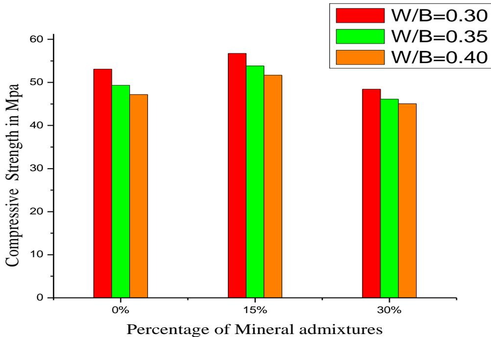
Figure 2: Compressive-strength for Partial replacement of cement with (0%,15%,30%) of mineral admixtures for 1% fibers (0.75% S.F & 0.25% P.F) for 7 days
