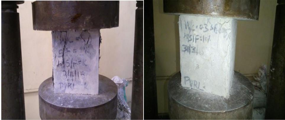
Figure 1: Schematic of compressive strength test
