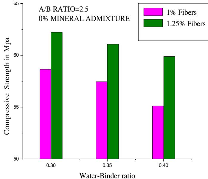
**Figure 7: Compressive-strength vs. Water-Binder ratio with different fibers percentage with 0% mineral admixture for 28 days**
