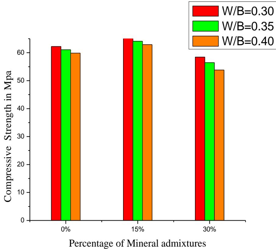
Figure 5 Compressive-strength for Partial replacement of cement with (0%,15%,30%) of mineral admixtures for 1.25% fibers (1% S.F & 0.25% P.F) fibers for 28 days
