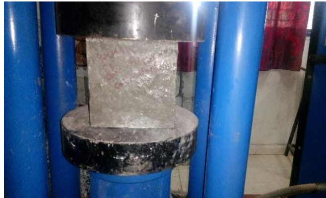
Figure 7: Lab testing of cube specimen
