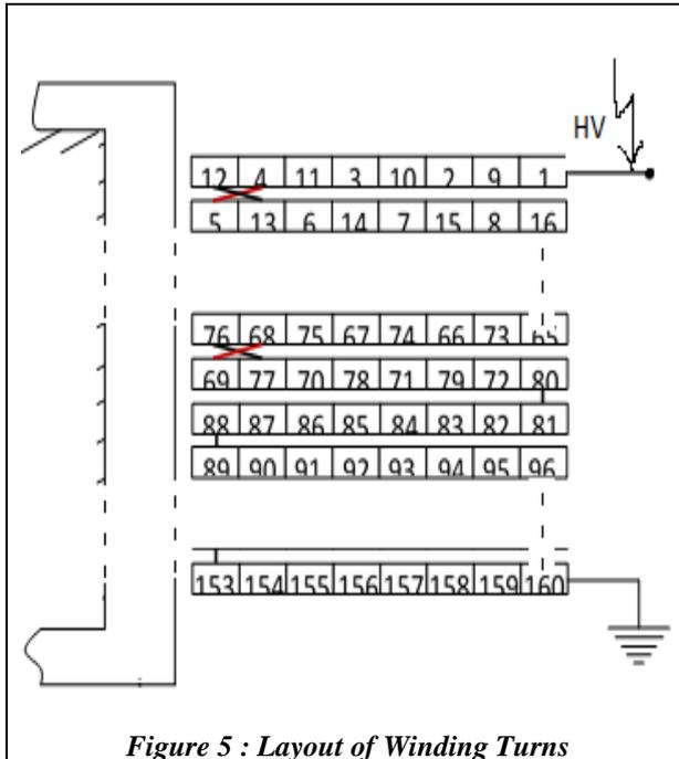
*Figure 5 : Layout of Winding Turns*
