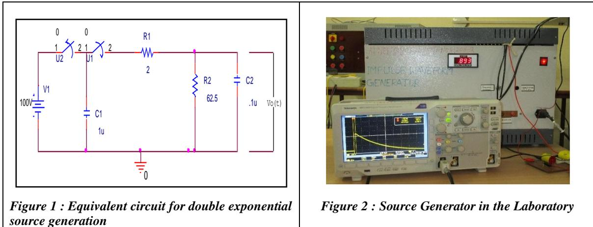
Figure 1 : Equivalent circuit for double exponential source generation
