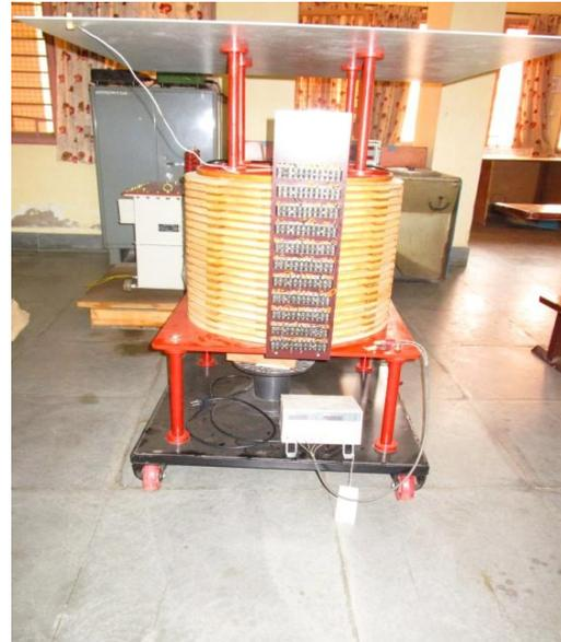
*Figure 6 : Air cored Transformer winding Model*
