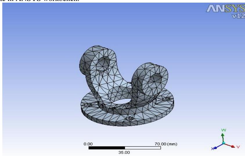
**Figure 5 Meshed model of universal joint yoke in ANSYS workbench**
