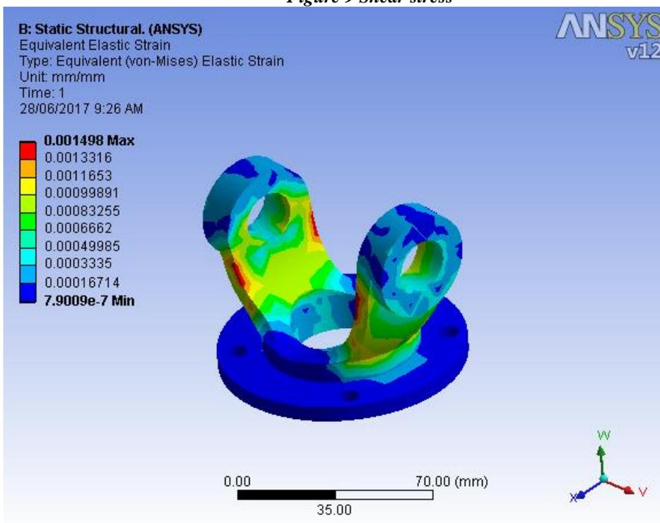
Figure 10 Equivalent elastic strain
