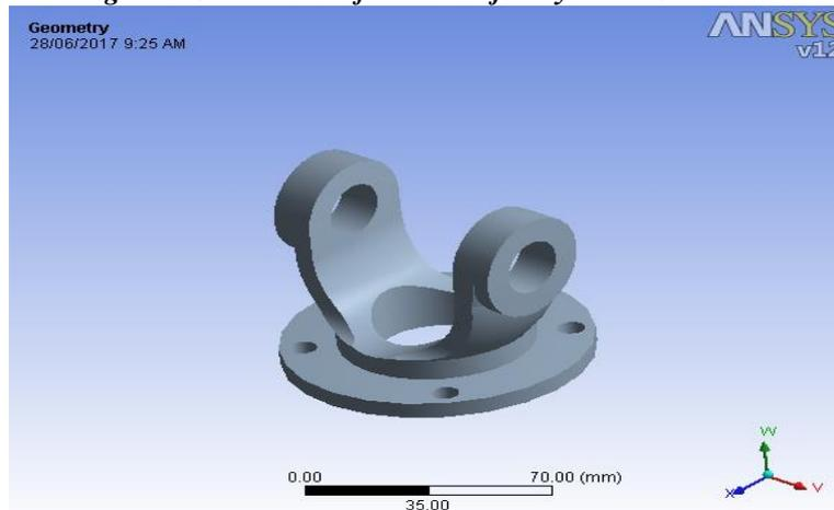
**Figure 4 CAD Model of universal joint yoke in ANSYS workbench**
