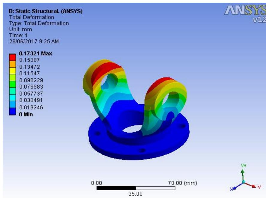
Figure 8 Total Deformation
