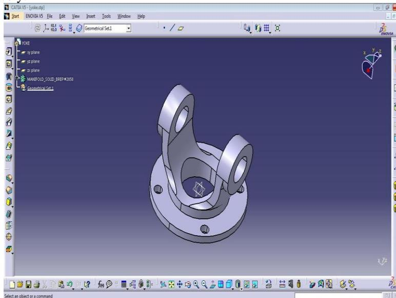
**Figure 3 CAD Model of universal joint yoke in CATIA V5**
