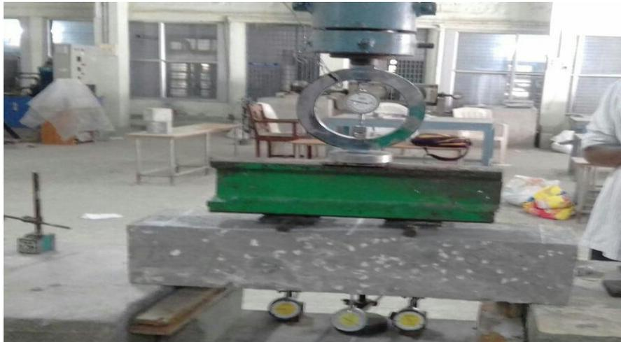
**Figure 2: Flexural Testing Machine**
