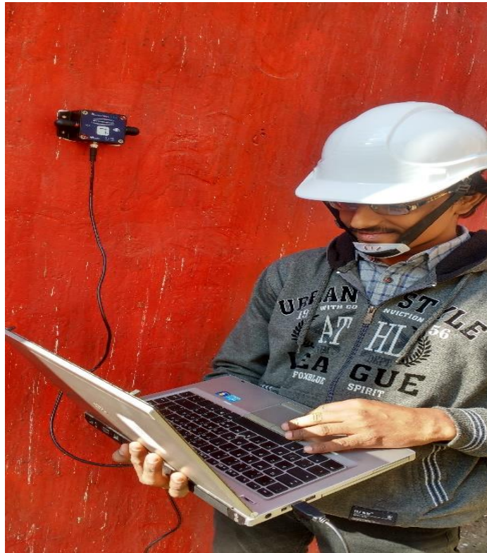
Figure 5. Collecting data using inclinometer sensor
