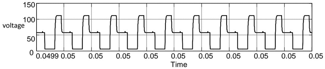
**Fig.12. Secondary Transformer voltage of Tr2 at voltage  $V_{rec}$**
