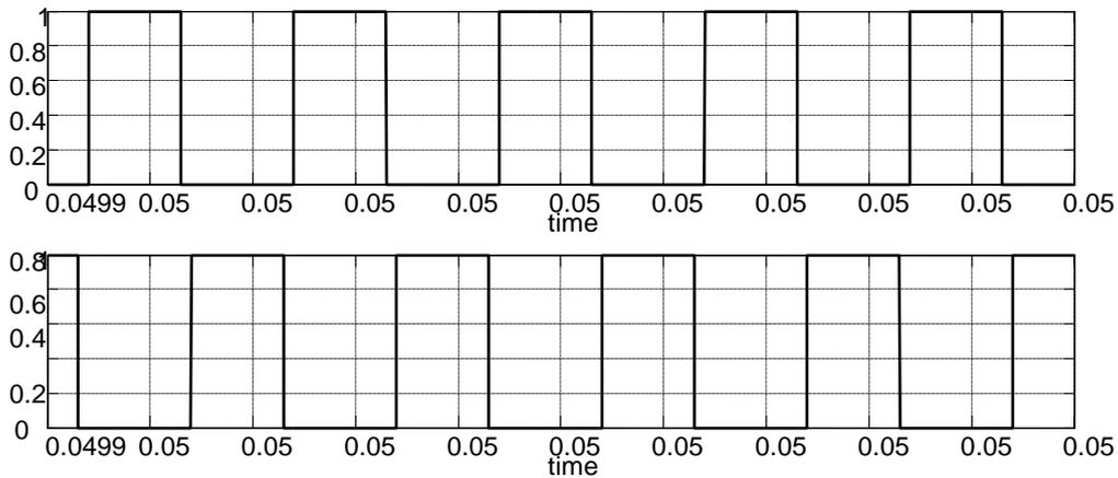
Fig.5. Gate Switching pulses of Q2,Q3
