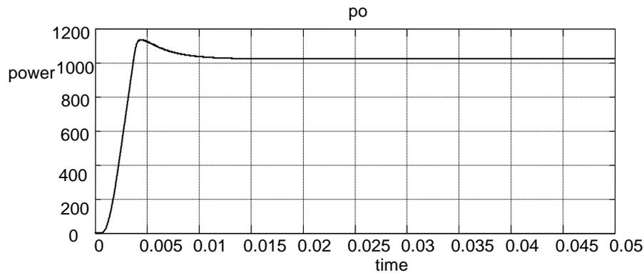
**Fig.15. Proposed Converter Output Power Vs Time**
