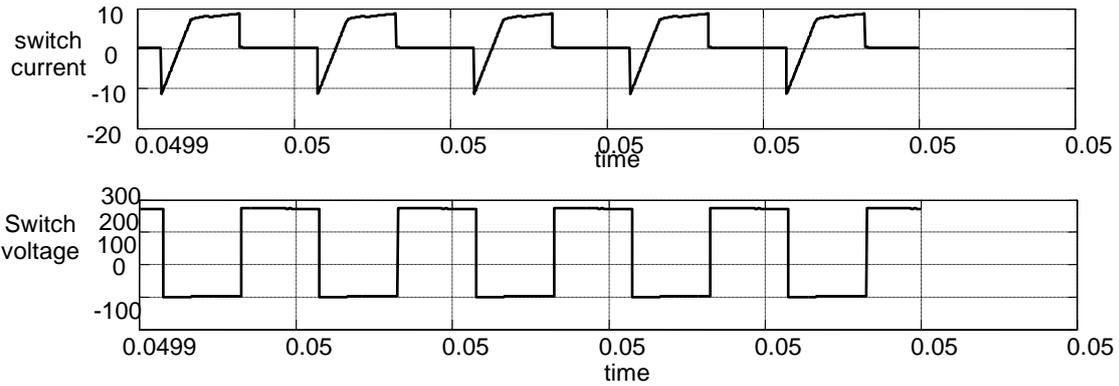
Fig.7. ZVS Of Q2 switching current and voltage
