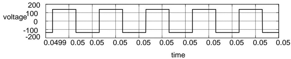
**Fig.13. Primary Transformer voltage of Tr1 at voltage  $V_{ab}$**
