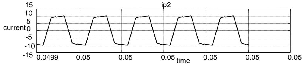
**Fig.11. Primary transformer of Tr2 current at  $I_{p2}$**
