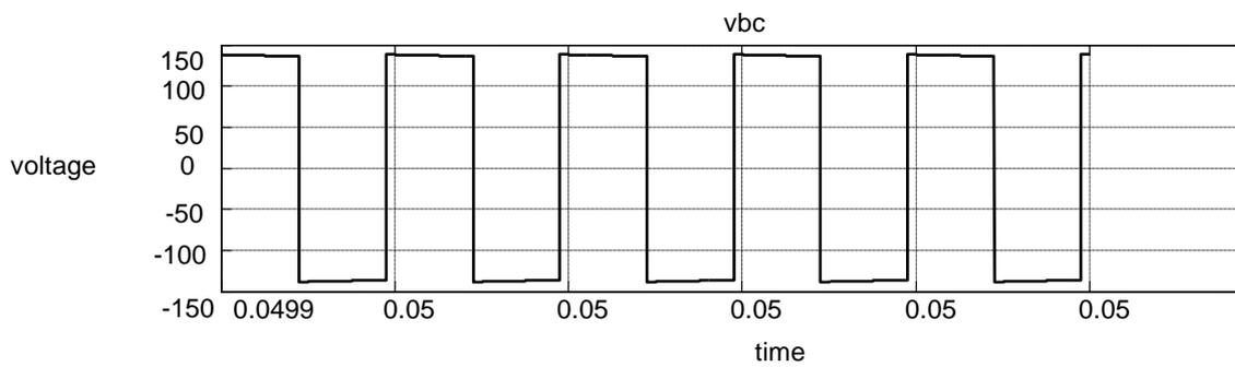
**Fig.14. Primary Transformer voltage of Tr1 at voltage  $V_{bc}$**
