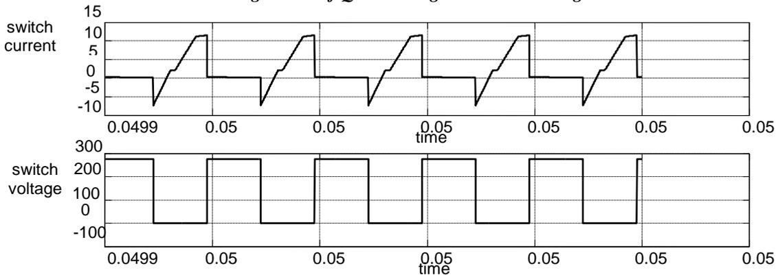
Fig.9.ZVS Of Q4 switching current and voltage
