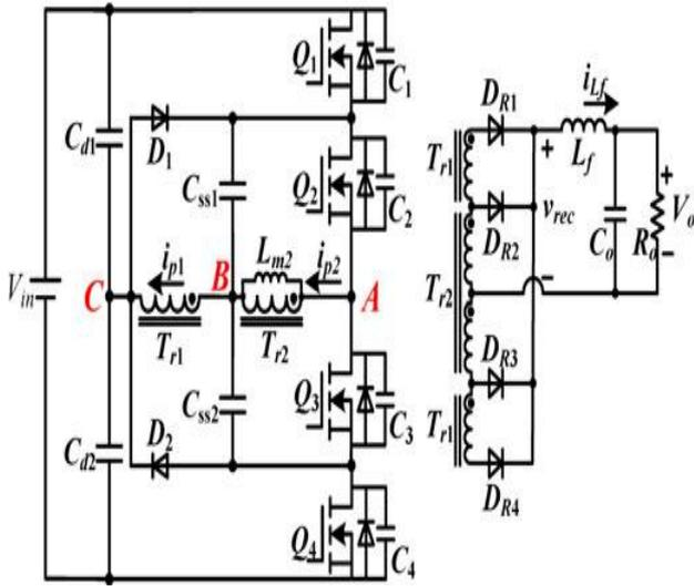
Fig. 1. Proposed Two Level HB converter
