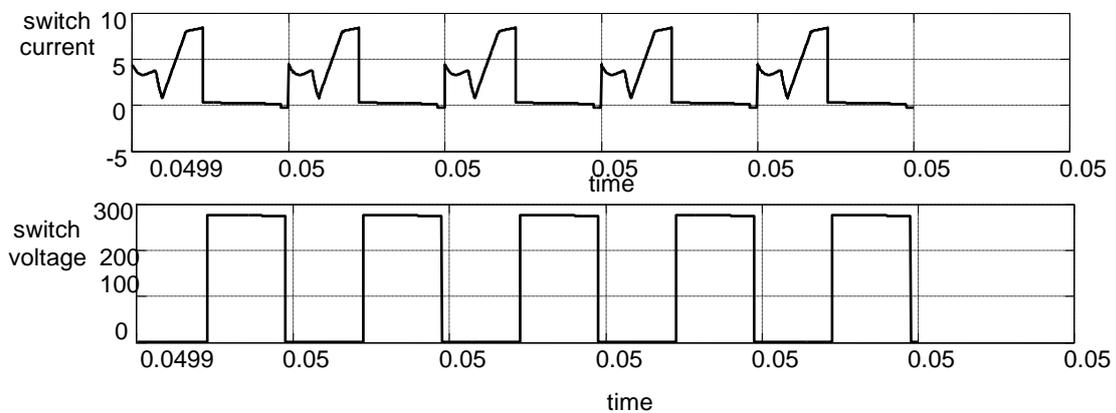
Fig.6.ZVS Of Q1 switching current and voltage
