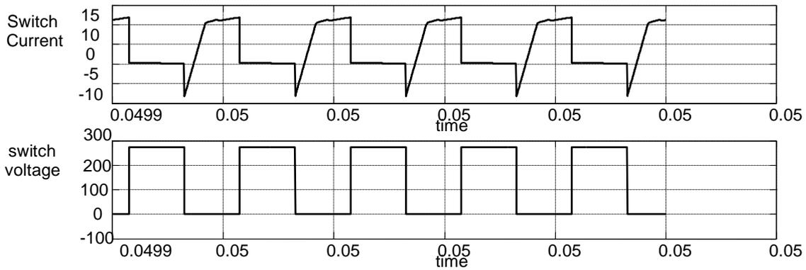
Fig.8.ZVS Of Q3 switching current and voltage
