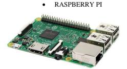
"The Raspberry Pi is a low cost, credit-card sized compute that plugs into a computer monitor or TV, and uses a standard keyboard and mouse. It is capable little device that enables people of all ages to explore computing, and to learn how to program in languages like scratch and python."
