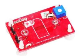
Heart beat sensor is intended to give advanced yield of warmth beat when a finger is put on it. At the point when the heart beat identifier is working, the beat LED flashes as one with every pulse. This computerized yield can be associated with miniaturized scale controller straightforwardly to quantify the Beats every Minute (BPM) rate. It takes a shot at the rule of light adjustment by blood move through finger at each heartbeat.
