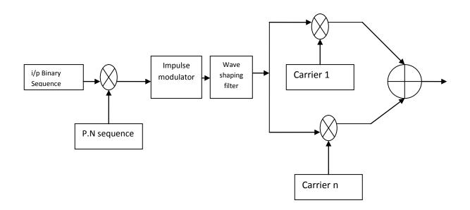
Block diagram of transmitter
