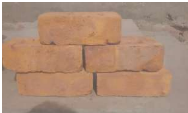
Fig.5. Brick of waste soil remains from stone industries
