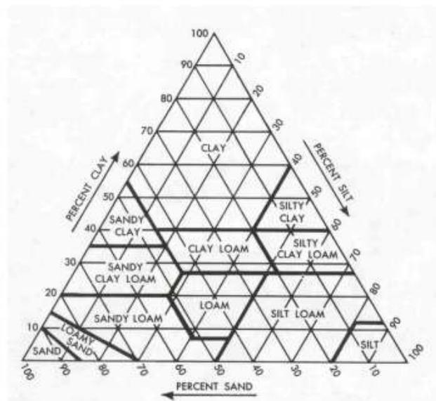
Figure 1: USDA Soil Triangle Classification Chart (The Asphalt Institute, 1978).
