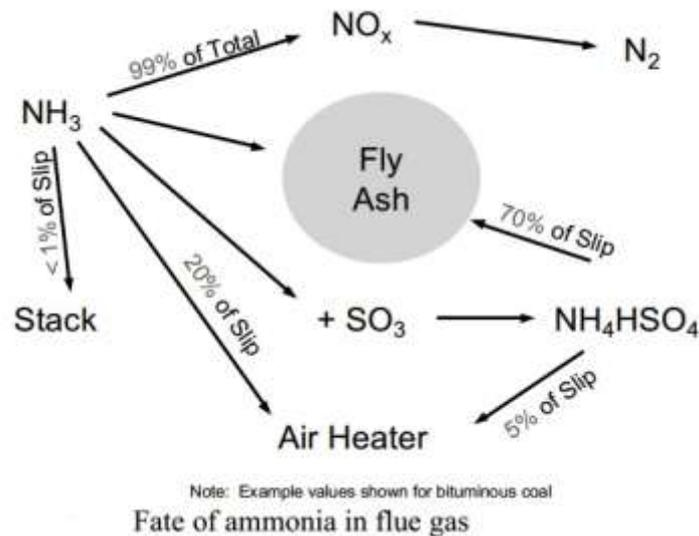
Figure 4: Ammonia Deposition Mechanisms on Coal Ash
