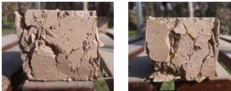
Figure 4 and 5: Specimens after compression tests
