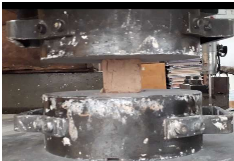
Figure 2: Cubic specimen placed in UTM for compression test
