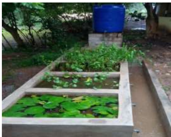
Figure 2: Constructed Wetland System setup with vegetation growth after two months of study
