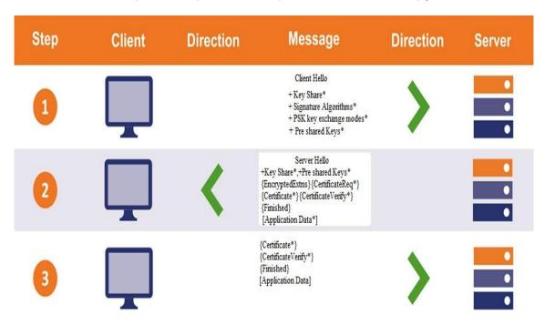
Figure 1. Message flow for full TLS handshake
