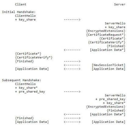
Figure 2. Message flow for resumption and PSK
