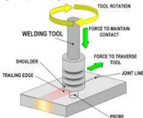
Figure 1: Friction Stir Welding Principle [1]
